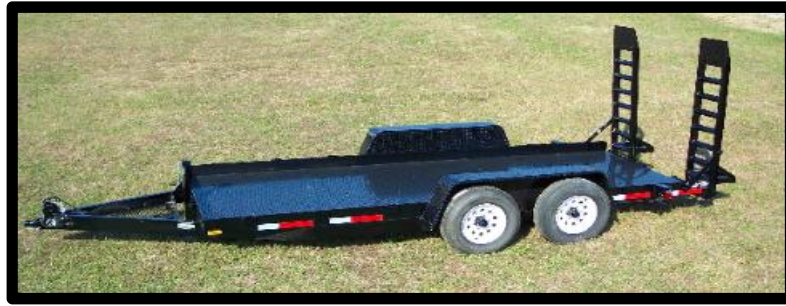
Trailer Shown with Heavy Duty 5' Ramps & Steel Floor Option
